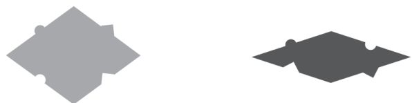
FIGURE 2 Penrose tiles consist of two shapes, which create patterns with a 5-fold symmetry—an interesting, if tricky to manage alternative to squares and hexagons. In this case, two rhombus shapes make tiling with a star pattern at the center. The markings on the edges indicate matching sides.
